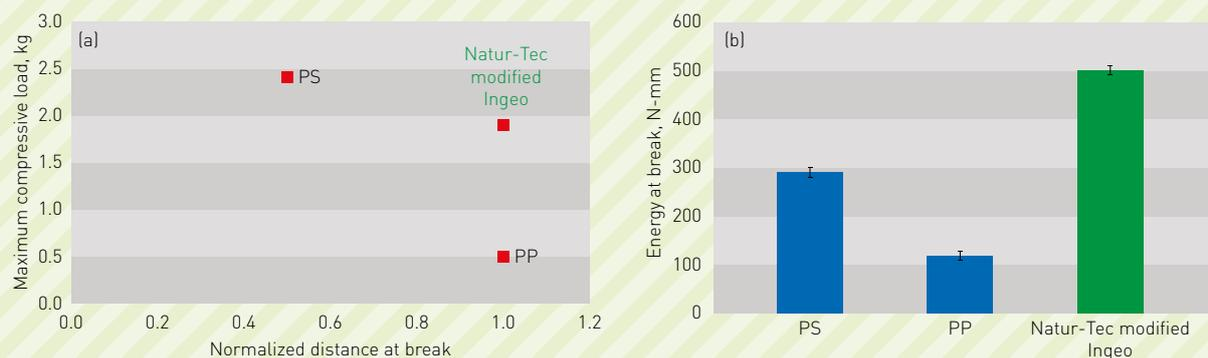
Figure 3: Hot water performance of spoon made with PS, PP and Natur-Tec's modified Ingeo PLA (a) at 80 °C and (b) at 90 °C
